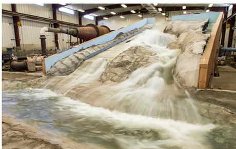
*1:50 scale model of the damaged Oroville Dam spillway built at the Utah Water Research Laboratory.*
