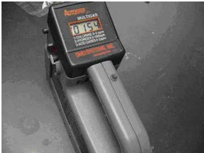
Figure 1. Portable paper-tape monitor used to measure arsine gas
