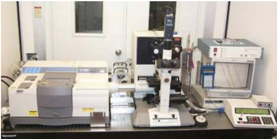
Synchrotron-based FTIR microscope at the Lawrence Berkeley National Laboratory Advanced Light Source that is being used to monitor bacterial contaminant degradation
