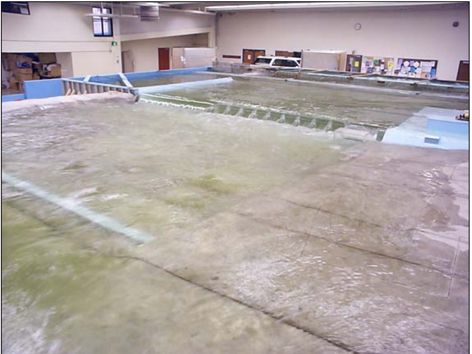
Another view of the Miller Dam Model at the UWRL
