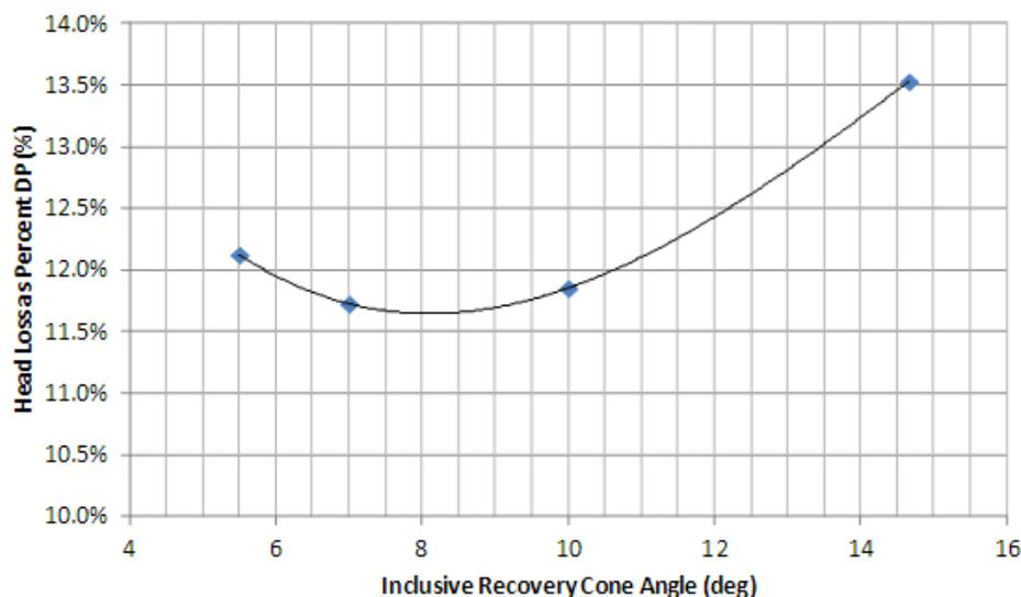
*Head loss versus cone angle for a 0.6 beta ASME Venturi with surface roughness. This plot shows that the meter design with the 7 degree recovery cone has the least head loss of the designs tested and that an 8 degree recovery cone would be optimal.*
