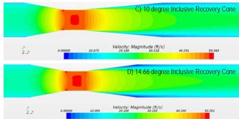
*CFD velocity contour plots showing some different recovery cone angles tested during the research. Can you guess which design produces the least head loss?*
