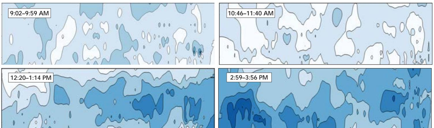
Ozone “curtains” or 2-D concentration maps extending WSW from Promontory Point, UT. Overall O<sub>3</sub> increased (darker) and pushed west as the day progressed. Late afternoon flights seemed to show increased O<sub>3</sub> at lower elevations over the GSL’s open water.
