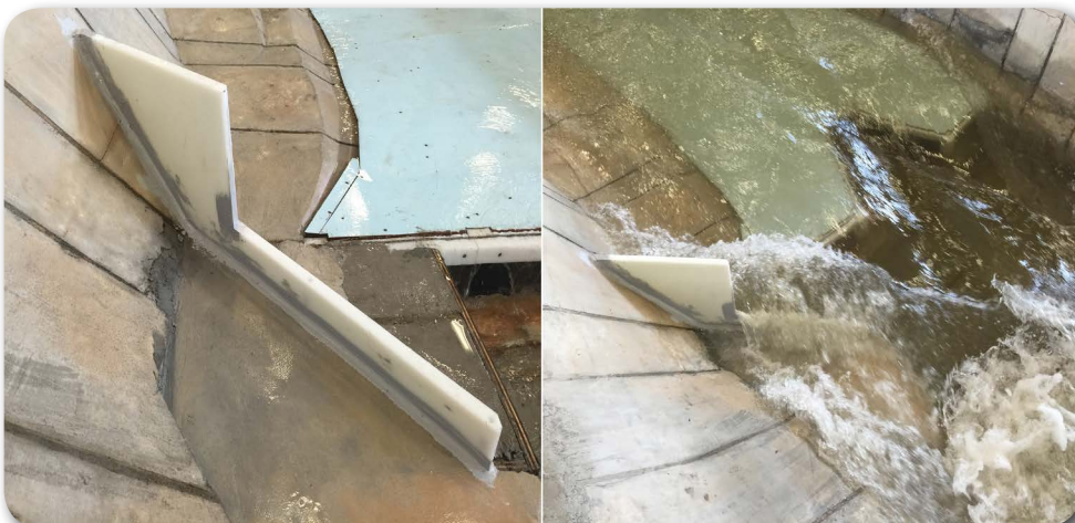
Physical and numerical models at the Utah Water Research Laboratory test the effectiveness of structural modifications to the Virgin River Gorge fish barrier
