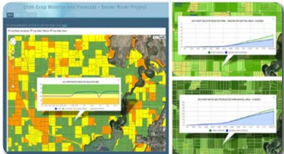
CWMIS layer maps of the Lower Sevier River Basin displaying (1) current and past crop water stress (left), (2) accumulated dry crop biomass in TM/acre (upper right) and, (3) accumulated crop water use in inches (lower right)
