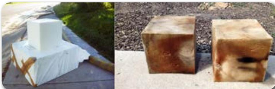
Foam swabs before and after passing through pipes
