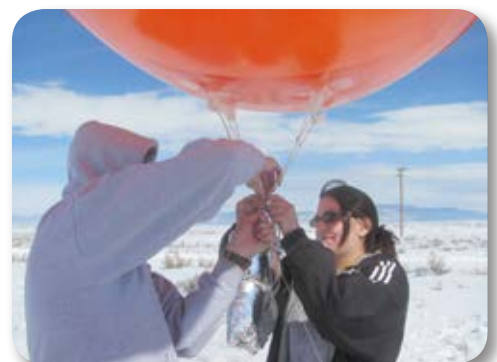
Researchers attach the air quality monitor system to a tethered balloon
