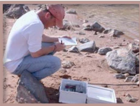
Ilan Gowin records solar radiation measurements within the water column
