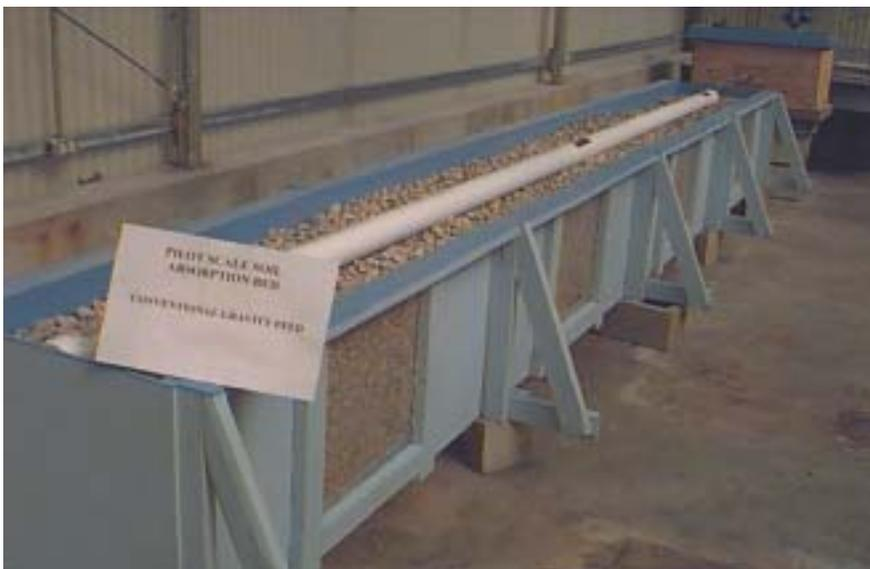
Pilot-scale soil absorption field trench
