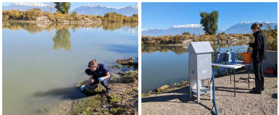
Figure 2: Water and aerosol sampling from Utah Lake for cyanotoxins (USGS 104B).
