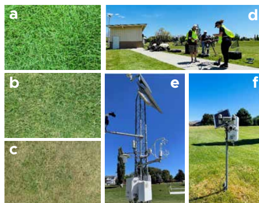
Figure 2: High (a), intermediate (b), and low (c) turfgrass quality, team preparing AggieAir drone for flight at Eagles Lake Golf Course (d), and eddy covariance surface energy balance system (e,f).
