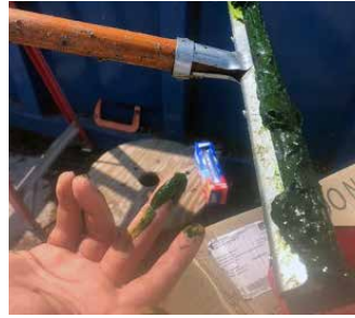
Figure 3: Harvested algae have a “paste” consistency when removed from the RABR using a rubber-bladed squeegee.
