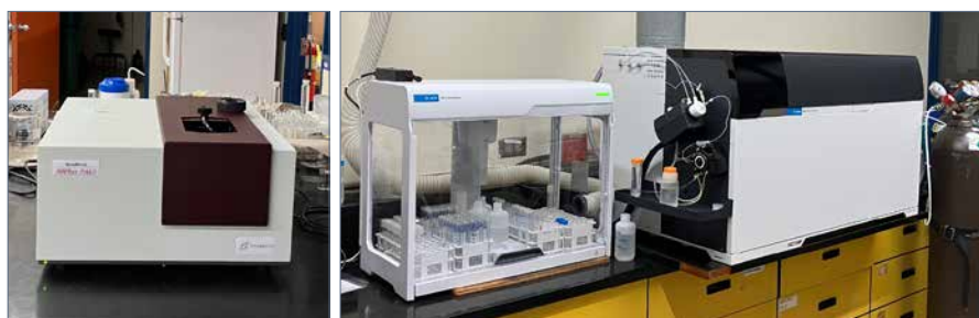
Figure 2: Recently purchased instrumentation to characterize (dynamic light scattering and zeta potential) and quantify (single particle ICPMS) NPs.
