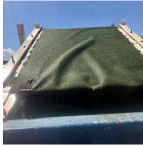
Figure 2: One RABR shelf with algae cultivated on recycled plastic support.
