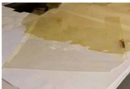
Figure 1: Sunlight-weathered polystyrene films showing yellowing with weathering and highlighting the effect of sunlight exposure.
