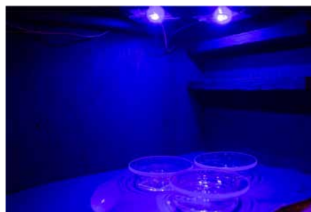
Figure 2: Ultraviolet light-emitting diodes used for aging plastic.
