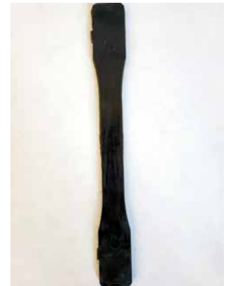
Figure 5: Bioplastic made from algae provided by Algix for biodegradation testing.
