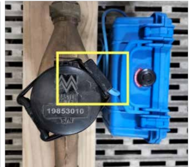
Horsburgh's custom datalogger (left), and the datalogger housed within the blue box and attached to a standard water meter (right). The connection to the meter is shown within the yellow rectangle.
