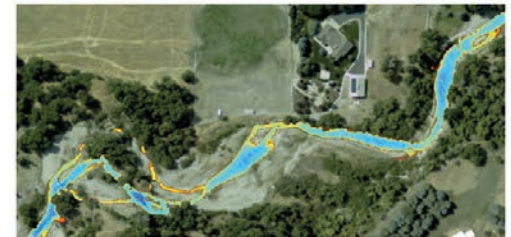
River instrumentation deployed between the Nibley Blacksmith Fork and Millville Providence Blacksmith Fork Lower canals over summer 2018. The UWRL's AggieAir™ UAVs were used to collect aerial and thermal imagery to assess spatial patterns of water temperature.
