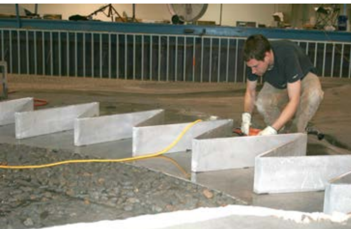
Construction and testing of the new 3150-ft long, 30-ft tall arced labyrinth weir emergency spillway (1:45 scale) for Isabella Dam
