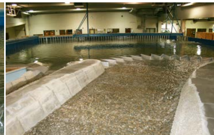
Construction and testing of the new 3150-ft long, 30-ft tall arced labyrinth weir emergency spillway (1:45 scale) for Isabella Dam
