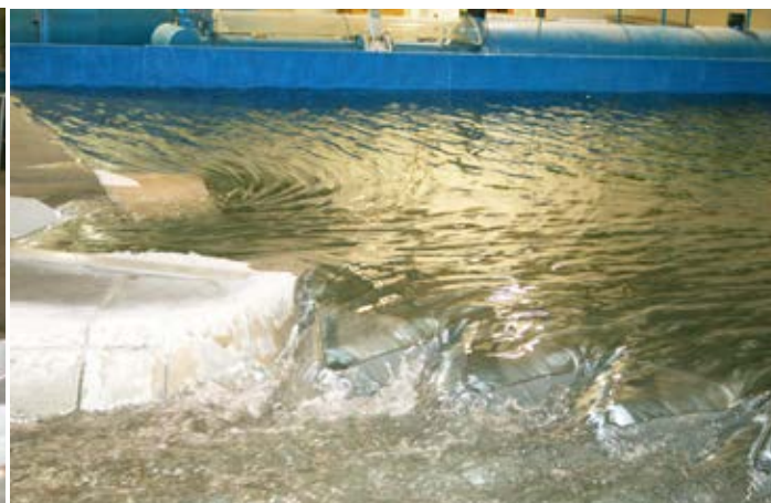
Construction and testing of the new 3150-ft long, 30-ft tall arced labyrinth weir emergency spillway (1:45 scale) for Isabella Dam
