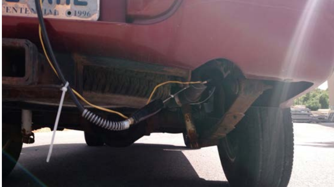
Vehicle equipped to measure emissions based on driver behavior and experience.
