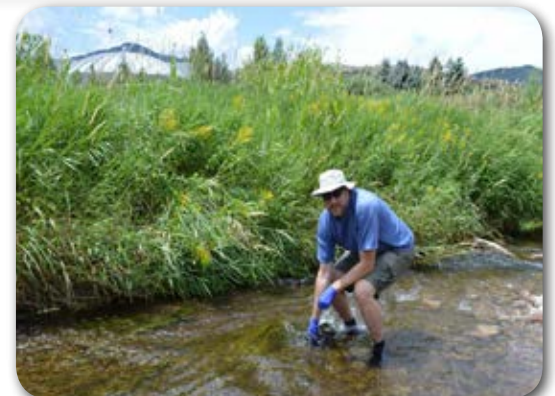
Collecting water samples in East Canyon Creek, Utah, to determine PPCP levels
