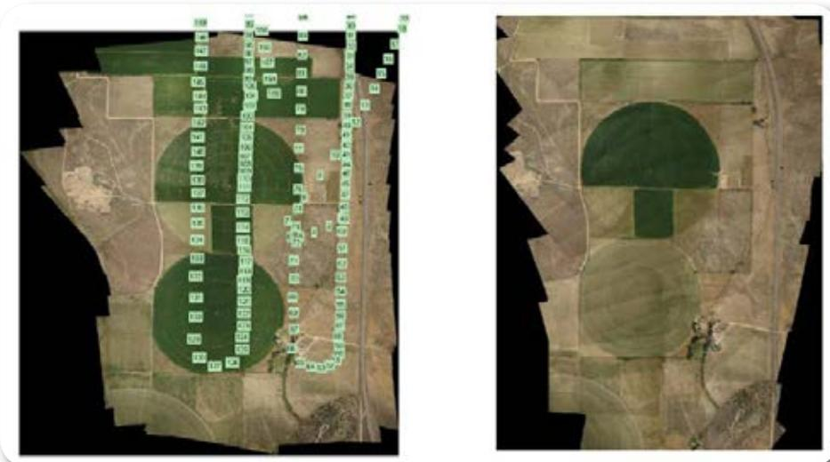
The base map and the obtained pixel locations for 158 aerial images using GPS information. The mosaic map generated by using the estimated pixel locations, the projective transformation, and the average of pixel values of the overlapping re-orthorectified images
