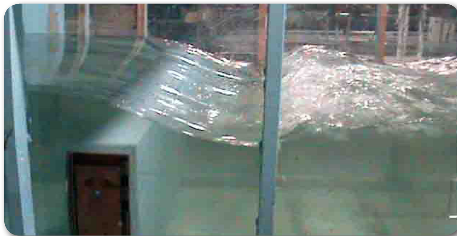
A physical scale model of a flat-topped low-head dam built at the Utah Water Research Laboratory to verify numerical model results and test remediation options
