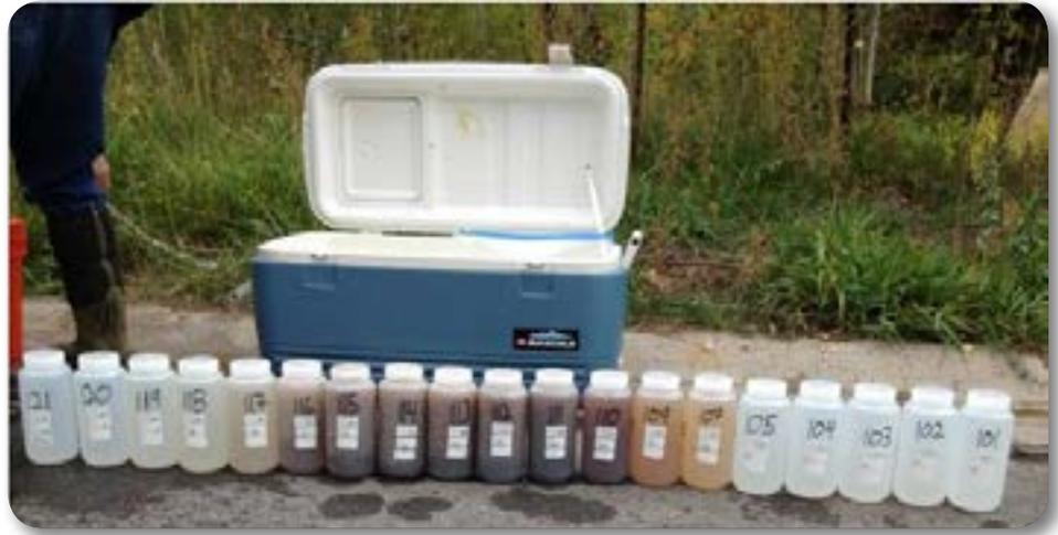
An array of water samples collected during an ice-pigging cleaning trial
