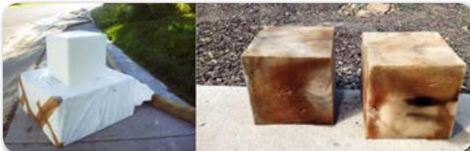
Foam swabs before and after passing through pipes
