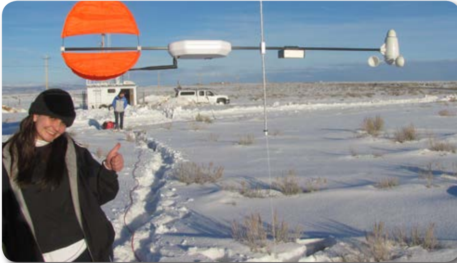
Crystal Wood prepares to deploy a tethered balloon used to measure ozone profiles
