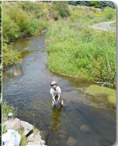
Collecting plant samples in East Canyon Creek, Utah, to determine PPCP concentrations
